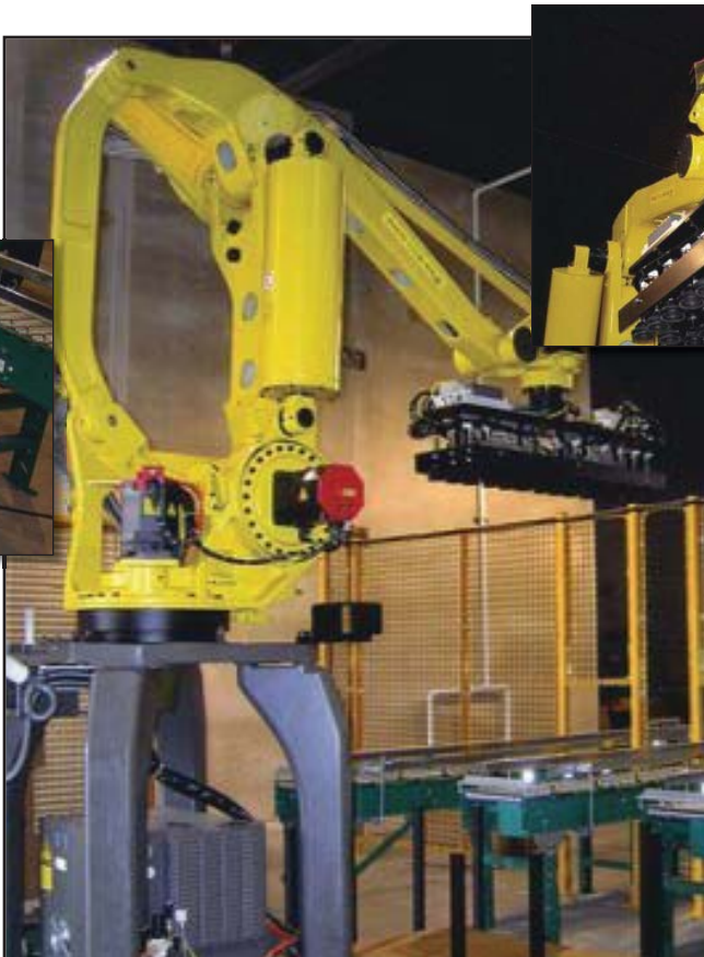
SMR SmartSTACKER™ selects from among up to four types of packed cases, presented on conveyors to assemble pallets with spacers, operating with precision according to a pre-programmed sequence and configuration of load.
